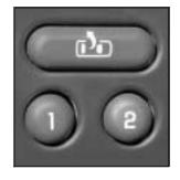
If your vehicle has this feature, the controls for the memory function are located on the driver's door.
